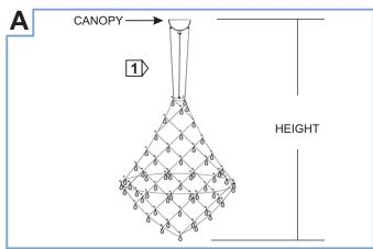
1: Determine the overall fixture height by adjusting the aircraft cable going into the canopy. Push the tab on the cord grip to release the aircraft cable.
